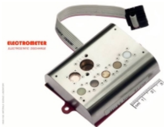
Figure 1. The MECA Electrometer showing five insulators over the triboelectric sensors (lower part), a bare electrometer (top left) and an ion gauge (top right).
